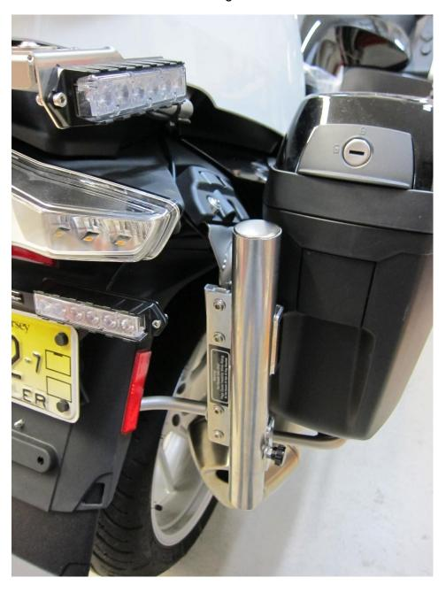
Attach the four M6 clip nuts to the RH saddlebag frame as shown in the photo at right.
