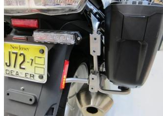
Bolt the flag pole mount to the four clip nuts using the M6 washer-head Torx screws provided using a T30 driver. You may wish to apply a small amount of antiseize compound to the threads of the bolt to prevent gauling – particularly if the mount will be removed and reinstalled periodically.
